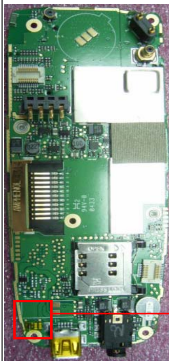
Add insulator tape on MB P/N: 76H00759-00
