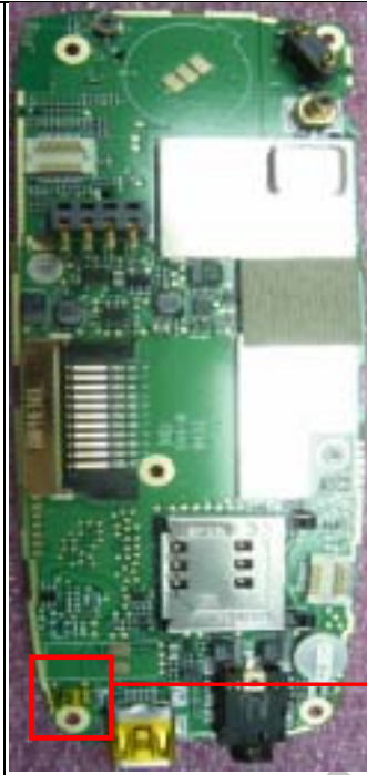
Add insulator tape on MB P/N: 76H00759-00
